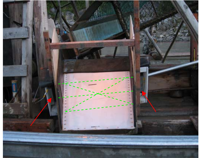
Infrared transmitter / receiver placement (red), and direction of beams across chute (green).
