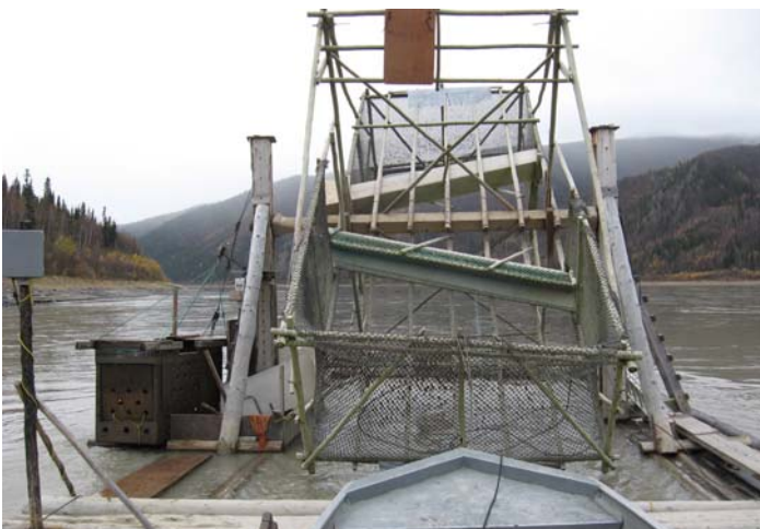
Video wheel pushed down river to be pulled out by winch at end of season.
