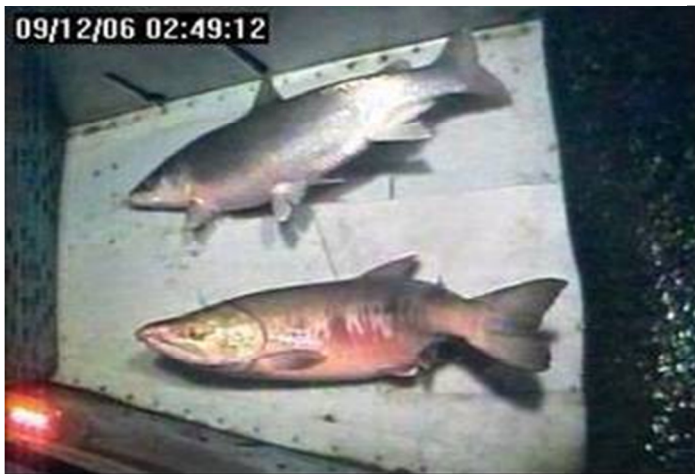
Infrared triggered LED testing light going on as fish pass sensor in slot mid chute (by sheefish) dorsal fin).
