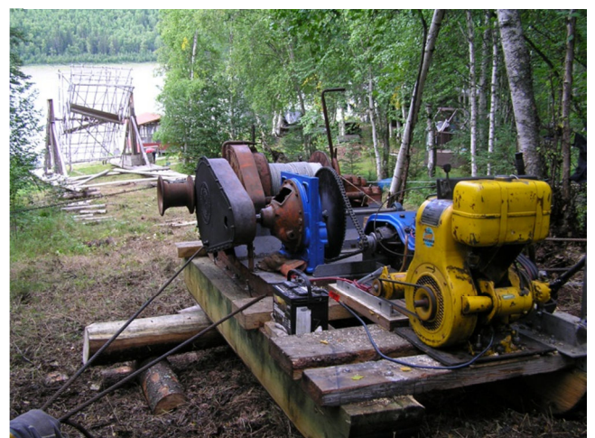
Winch used by project to move wheel in and out of water at Rapids in 2012
