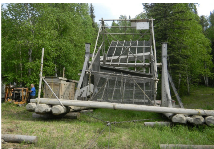
2012 Video wheel ready to be pulled in water by winch at Rapids.
