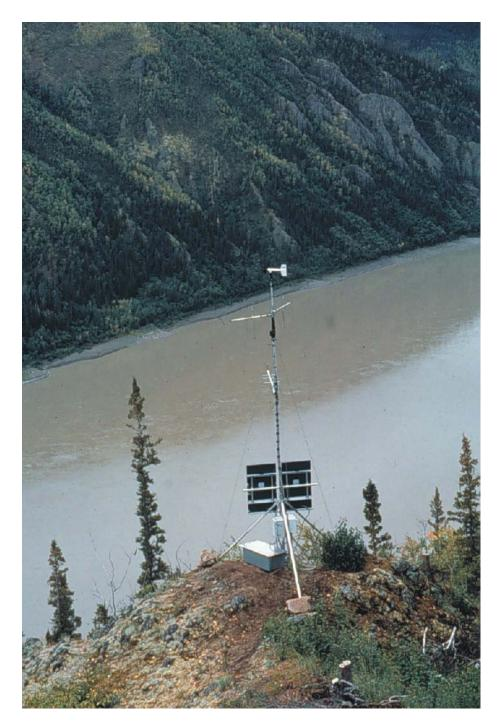
FIGURE 16.—Remote radio receiving station located on a high bluff over the Yukon River, 11 km upstream of the study site. This station, and others like it, recorded the passage of radio-tagged inconnu moving along the river.
